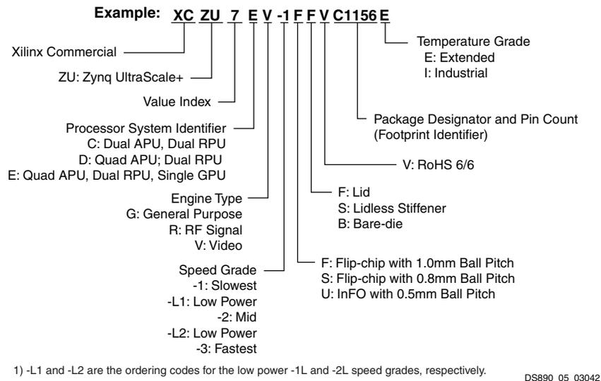
Figure 5: Zynq UltraScale+ MPSoC and RFSocC Ordering Information
